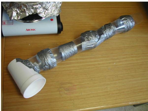
Here is the distiller, made of a styrofoam cup, plastic cups, and duct tape.
