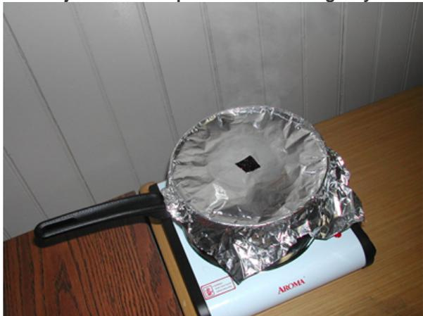
First, to aid in the containment of the steam, a piece of aluminum foil was placed over the top of the pot, and a hole was cut in the center. The distiller is placed over that hole.
