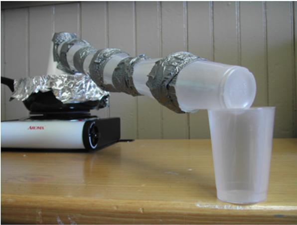
Each cup has a hole cut into its bottom so that the condensed water can trickle down.
